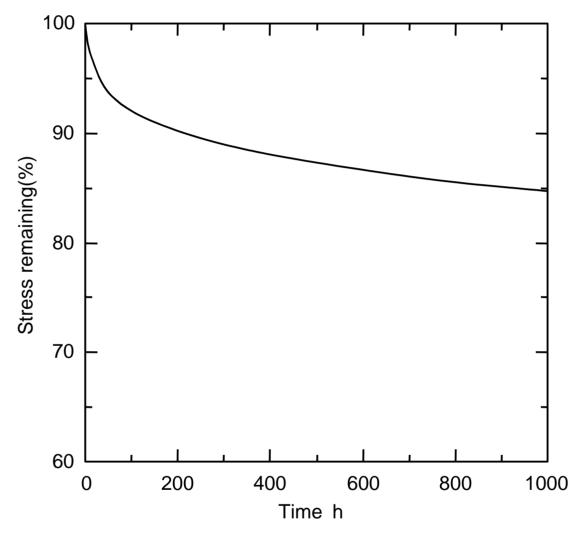
Fig.6 Stress relaxation of connector alloys at 150 .
